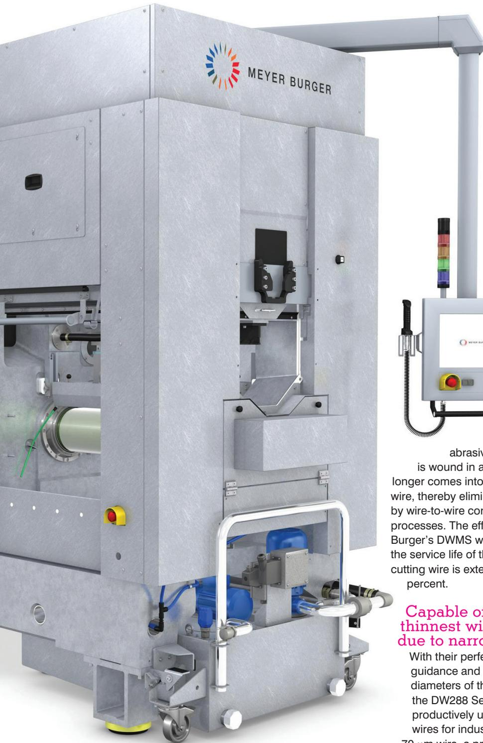
More and thinner wafers in a shorter time and with a lower consumption of diamond wire: Meyer Burger's DW288 Series 3 diamond wire saw combines a patented wire management system, optimized distances and diameters of the wire guiding rollers, and a consistently optimized automation, to create a highly productive overall package with a secure future.
